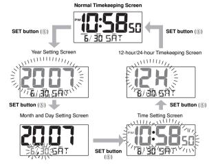
2. While the screen you want is on the display, use the Alarm Time Set buttons (4) to change the digits that are
